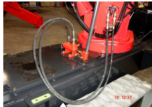
Illustration 5 showing crane ready for emergency winching
